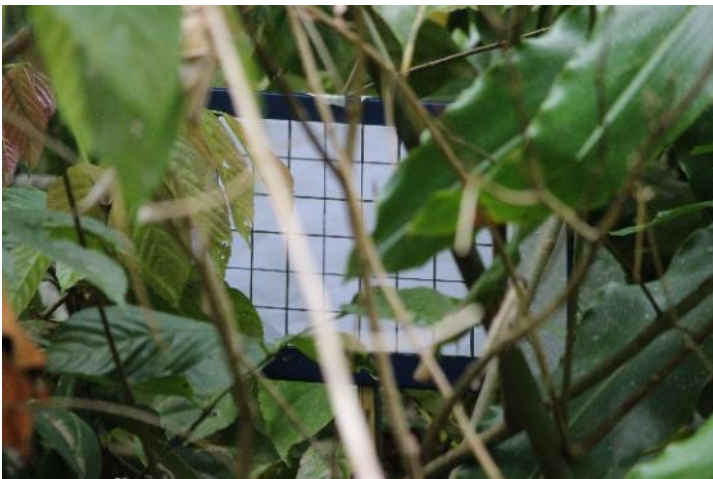
Figure 3. Gridded A4 paper with 3 x 3 cm squares. Number of visible white squares determine the vegetation density.
